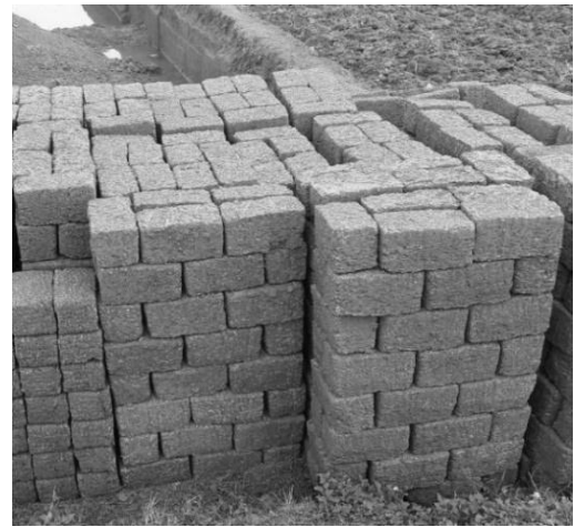
Fig. 6: Laterite bricks are dried before using
